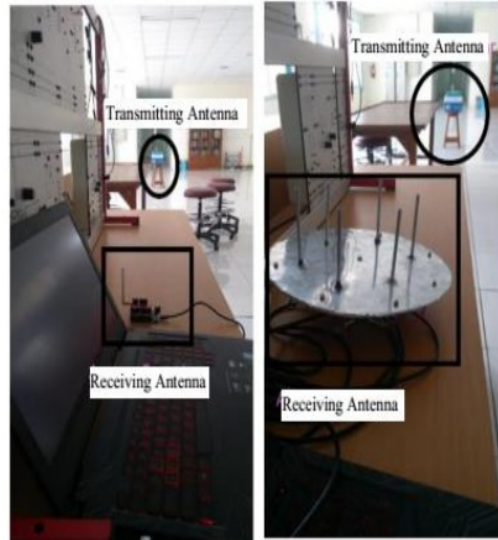
Figure 9. The measurement configuration set-up in the indoor 915 MHz IoT network environment
